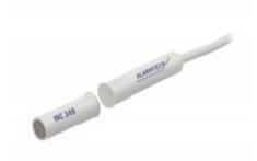
MC 346 is a universal magnetic contact with change-over (NC/NO) function that can be used in both alarm and access control systems for monitoring e.g. doors and windows against unauthorized opening. Both the contact and the magnet part are in a water proof (IP 67) plastic housing, which enables easy installation into wood without additional accessories. With our extensive range of installation accessories it is easy to install the contact either recessed or as a surface mount.
